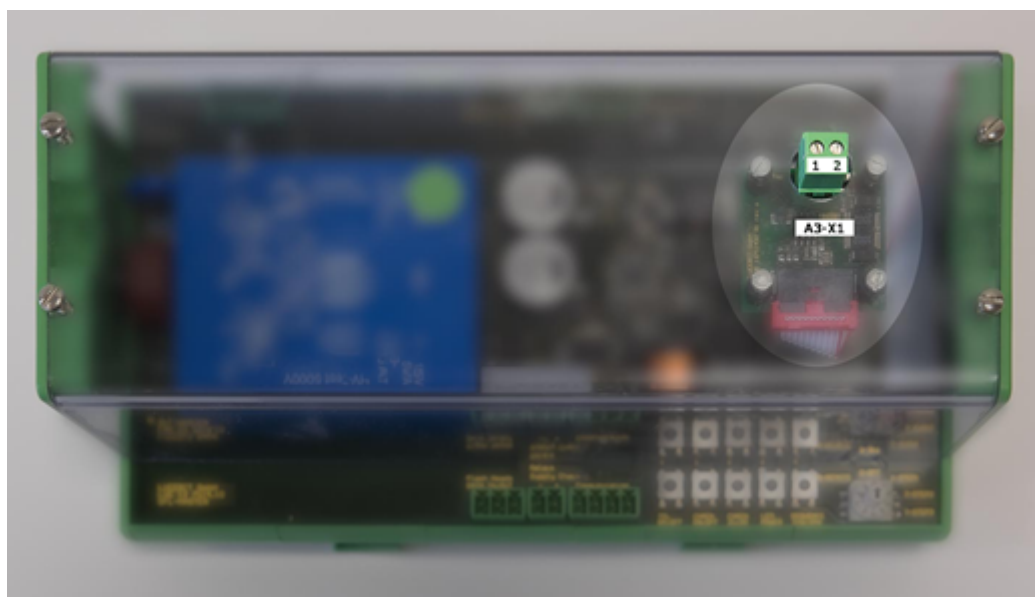
Figure 23: External trigger input on the control module
