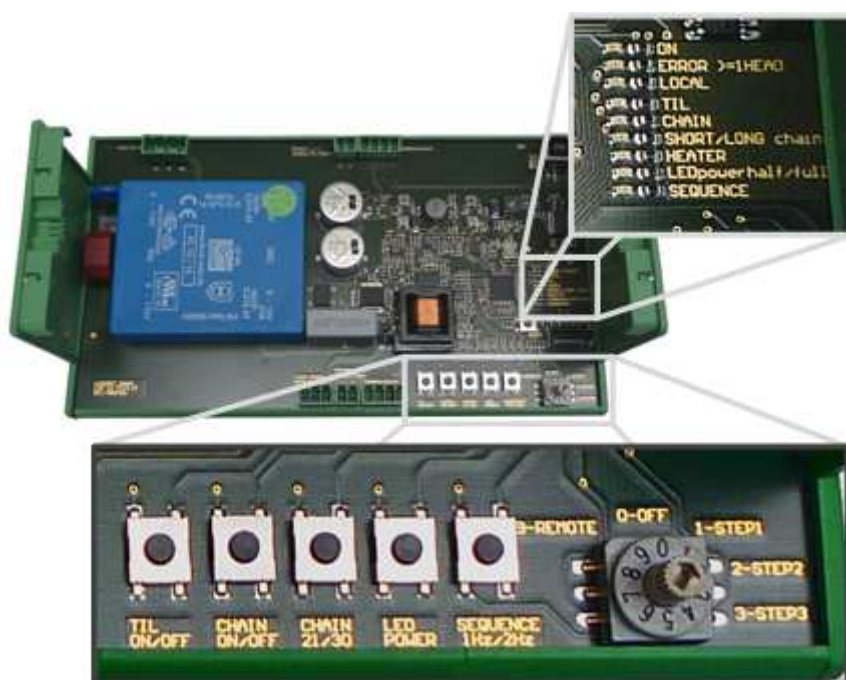
Figure 4: Service, operator control and display elements at the control module
