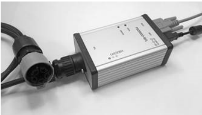
Figure 15: Parameterizing adapter for the settings of an inset flashing light
