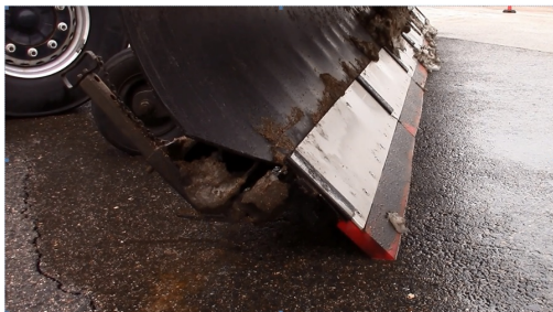
Figure 34: Fig. 1 — Snowplow blade with well aligned segments
