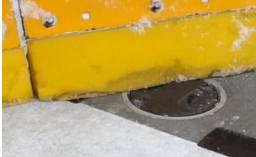
Figure 36: Fig. 3 — Snowplow blade without clearance
