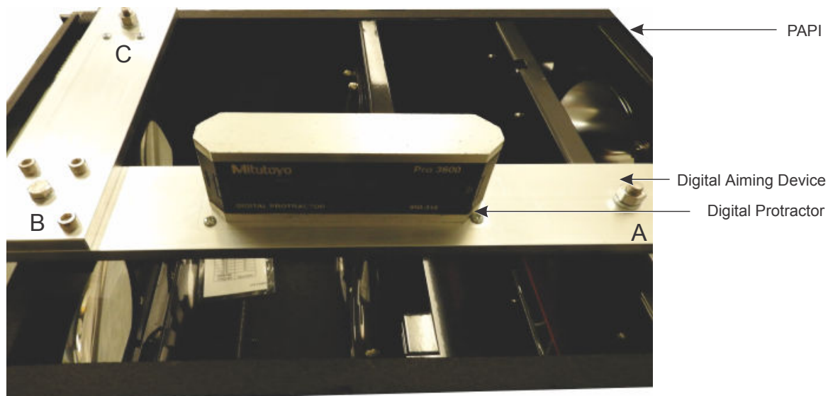
Figure 9: Side View of Digital-Level Aiming Device for Two-Lamp PAPI
