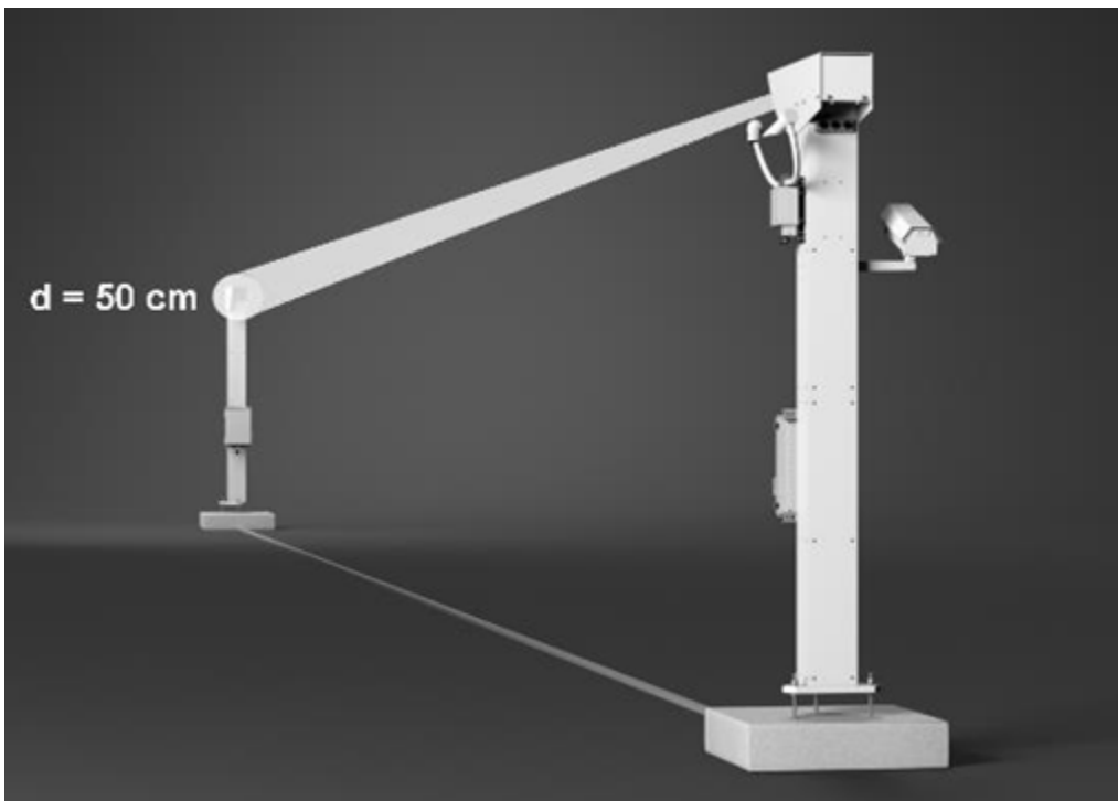
Figure 59. Center Light Beam from Transmitter on Receiver Head
