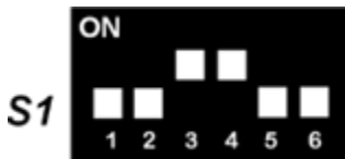
Figure 65. Control Board DIP Switch Settings for the M482306-00 Present Weather/Visibility Sensor
