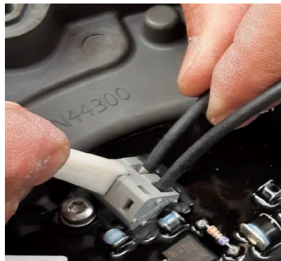
Figure 25: Releasing/locking secondary wires with insert tool
