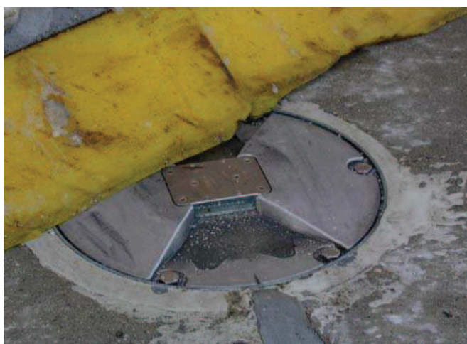
Figure 45: Signs of wear on plastic cutting edge
