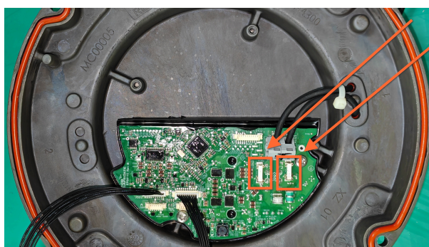
Figure 13: 1-connector converter (2 fuse resistors)
