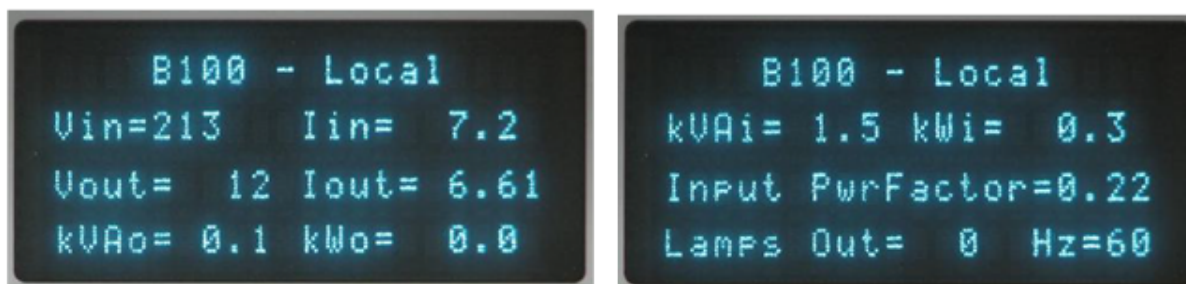
Figure 11: Displays - Additional Data Shown By Scrolling Down
