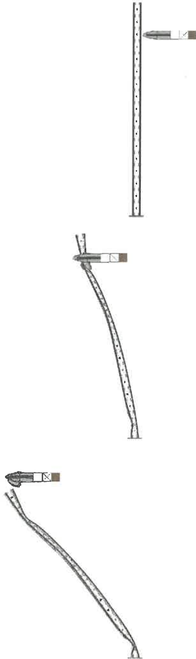
Figure 9: Deformable wing impacting the 4.9 m mast model at 0 ms, 40 ms and 80 ms.
