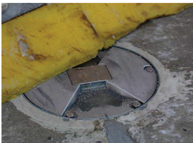
Figure 44: Signs of wear on plastic cutting edge
