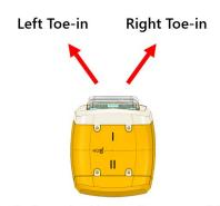
Toe-in determined by standing on top of the light fixture looking in the direction of the beam.
