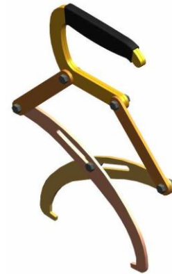
FIGURE 6 – LIFTING HOOKS TO REMOVE AND INSTALL LUMINAIRE FROM THE BASE RECEPTACLE
