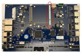
2. Assembly new heat bar with 2 screws M2,5x5 on back side of Carrier board
