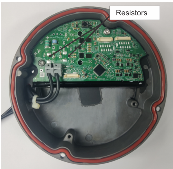
Figure 14: 1-connector converter (2 fuse resistors)
