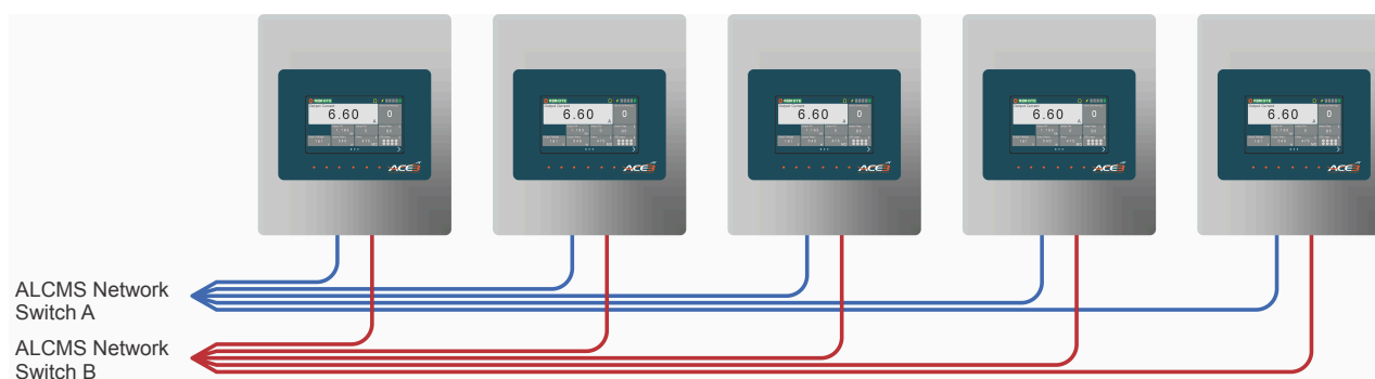
Figure 16: Redundant Ethernet Example
