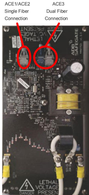
Figure 8: CVM2 connections
