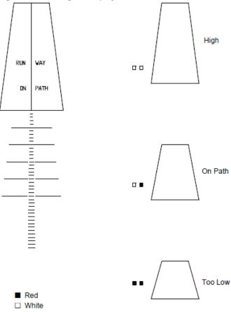
The units are aimed so that during a landing approach the pilot will see the following signal format:
