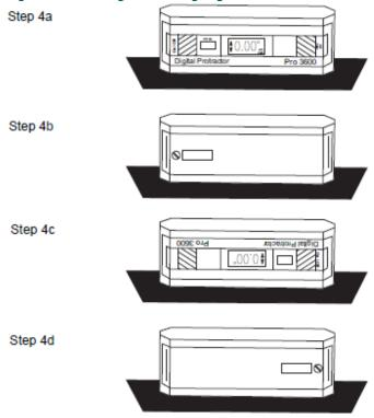
b. Rotate the digital protractor so that it faces away from you. The lettering should still be right-side up. Align with the same edge or line. Wait 10 seconds. Press the HOLD button until [2] appears.
