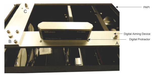
The two movable arms increase the stability of the aiming device and are used to establish the transverse horizontal references. Screws are provided on the bar and on the movable arms to guarantee an exact positioning of the level during setting and adjustment. This exact positioning is required to have a perfect match between the level and the longitudinal and transverse horizontal references. The two V-sights on the bar of the aiming device are for azimuth alignment.
