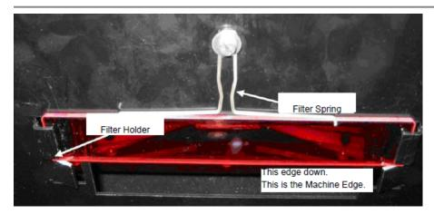
Each filter is held in place in the filter holder by two springs.
