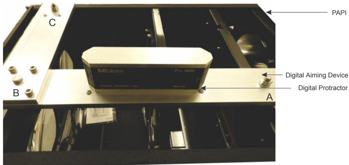
The two movable arms increase the stability of the aiming device and are used to establish the transverse horizontal references. Screws are provided on the bar and on the movable arms to guarantee an exact positioning of the level during setting and adjustment. This exact positioning is required to have a perfect match between the level and the longitudinal and transverse horizontal references. The two V-sights on the bar of the aiming device are for azimuth alignment.
