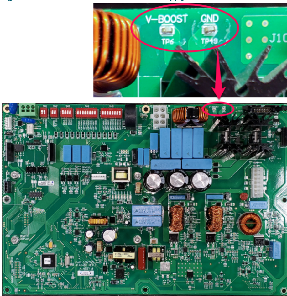
Figure 45: LED PAPI Control Board DC Power Supply Test Point
