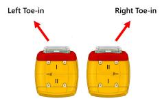
Toe-in determined by looking at the light fixture from the centreline.
