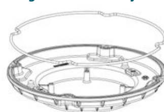
Figure 9 : Retirez le joint
