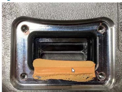
Figure 14: Removal of Deformed Orange Thermal Pad
