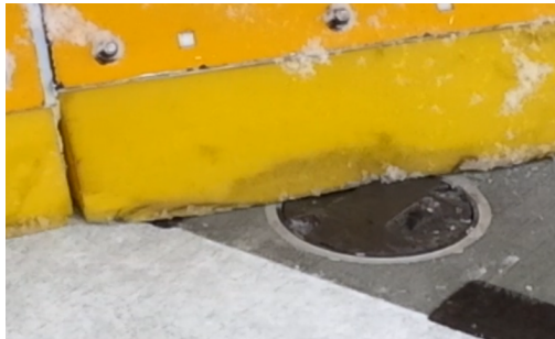
Figure 40: Fig. 3 — Snowplow blade without clearance
