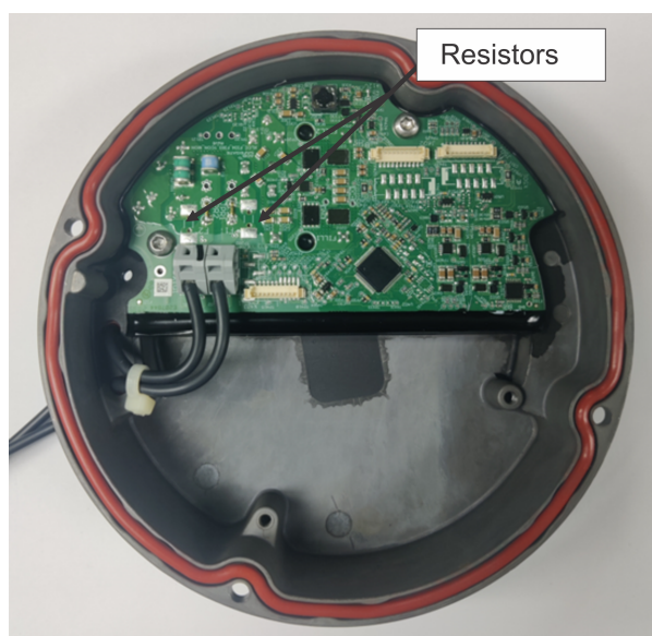
Figure 10: 1-connector converter (2 fuse resistors)
