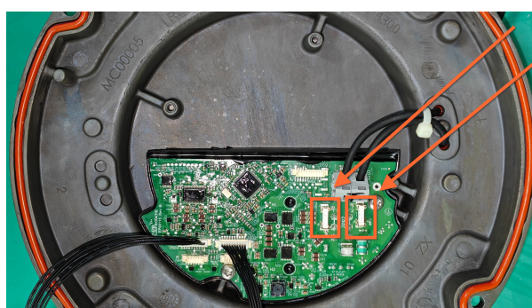
Figure 11: 1-connector converter (2 fuse resistors)
