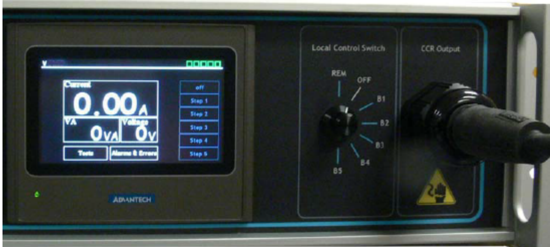
Figure 6: Circuit Breaker - ON with the Rotary Switch - OFF
