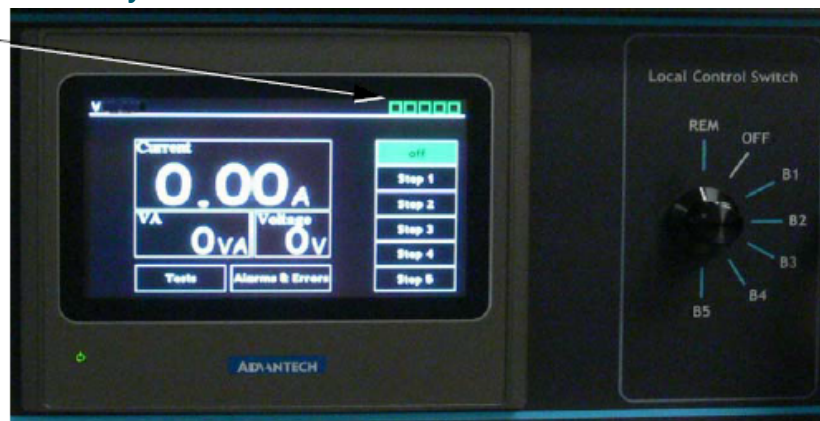
Figure 7: Circuit Breaker - ON with the Rotary Switch - Remote
