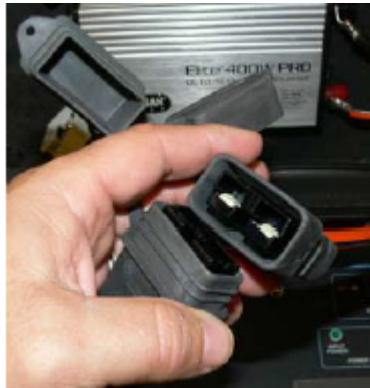
Power Inverter 12 VDC Coupling.
