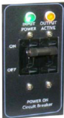
Figure 4: Circuit Breaker (Power ON) switch and Power Indicators
