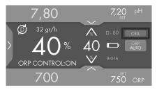
The electrodes are deactivated and it is necessary to replace them, "CELL" appears.See hours electrodes (5.5 Historical).
