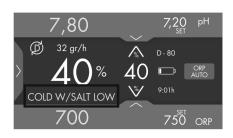
Low conductivity: cold water or low salt. The message "COLD WATER / SALT LOW" on display message bar also appears.
