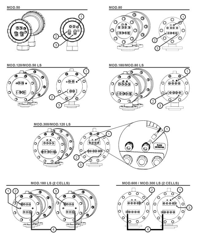
① Flow Detector ② Contact 1 ③ Contact 2 ④ Cable bridge between cells
