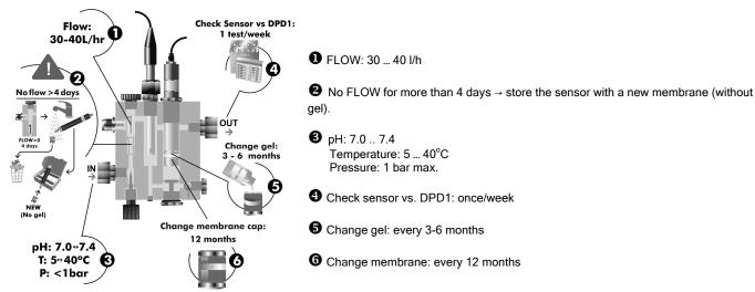
If calibration is not possible, because the reading is very low, then the sensor electrode [5] should be sanded with paper supplied in the installation kit (blue paper), and should also proceed to change the membrane and the electrolyte, as described below:
