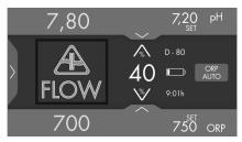
GAS: System is supplied with an integrated flow sensor based on detection of gas bubbles inside the electrolysis cell. This sensor allows to detect if there is sufficient water flow to ensure proper system operation. If flow is not enough, system will show "FLOW" alarm. See page 18.
