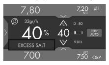
High conductivity: an excess of salt has been added. The message "EXCESS SALT" appears in the message bar of the display.
