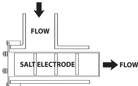
For the electrolysis chamber to work correctly, it is recommended that the heating system be placed within 20 m. of the pool (40 m. of back / forth piping).
