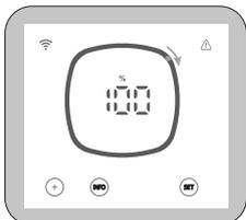
2. Model Ei2 iQ evo pH: cycles between current production (%) and pool pH.
