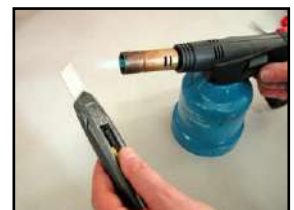
8. Heat the knife or cutter.
