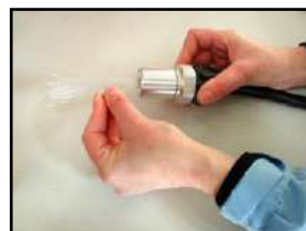
7. Hold the fibres with the packing gland and insert pieces of fibre until all the spaces are filled up.
