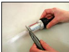
9. Rest the knife on the port and cut the projecting fibres.
