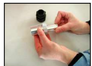
4. Insert the reducer inside the body of the optic port.
