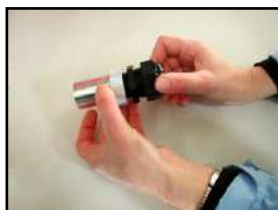
5. Screw the packing gland to the optic port.
