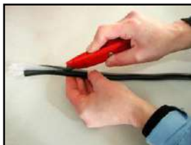
1. Cut approximately 10 cm. of the cable covering.
