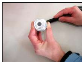
10. Polish the fibres with very fine sandpaper if they have been damaged when cut.
