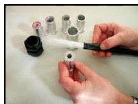
3. Choose the required reducer depending on the amount of fibres.
