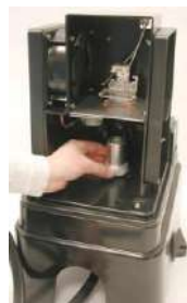
11. Insert the optic port through the openings located in the base of the generator and fasten to the clip.
