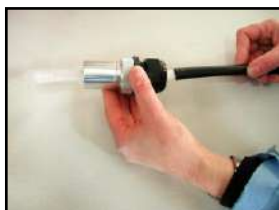
6. Insert the fibres in the port until they ALL come out of the port.
