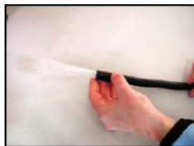
2. Check that the fibres are not damaged.
