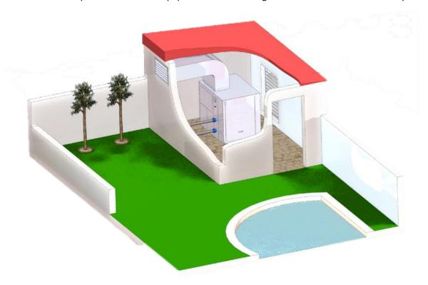
It is necessary to make the duct network so that the air collected by the machine to operate the refrigeration circuit, never return to the machine, and must be expelled to the street. The machine must be located exclusively inside.
