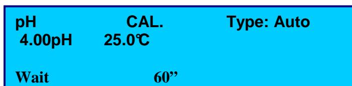
At the end of each calibration point, the instrument will display the quality of the electrode as a percentage.
