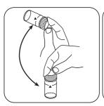
Dissolve tablet(s) by inverting.
