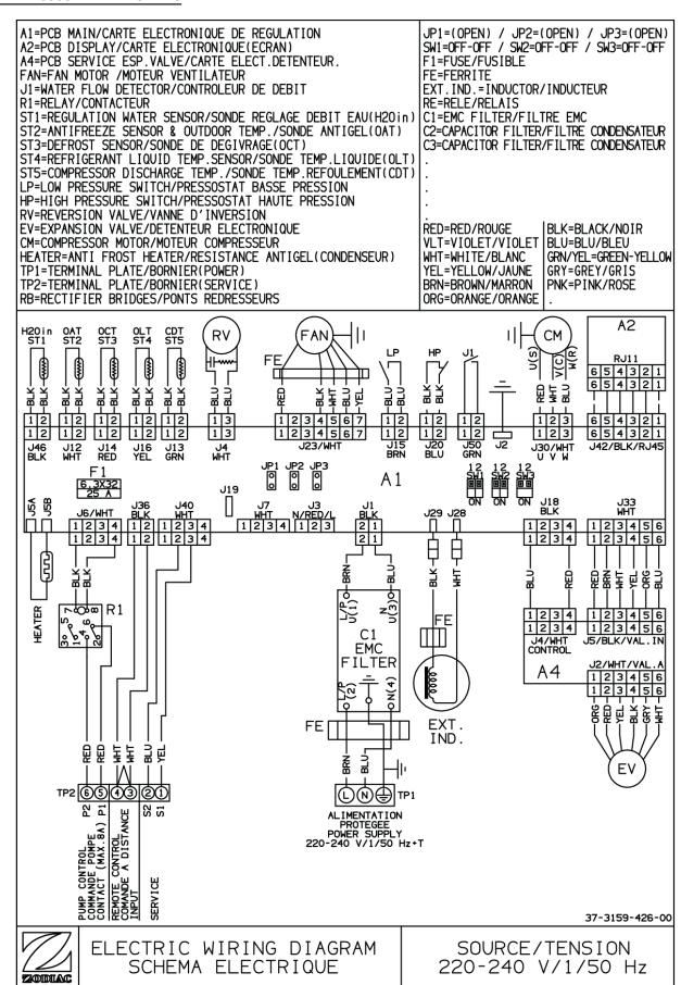
A1=PCB MAIN/CARTE ELECTRONIQUE DE REGULATION JP1=(OPEN) / JP2=(OPEN) / JP3=(OPEN) SW1=OFF-OFF / SW2=OFF-OFF / SW3=OFF-OFF A2=PCB DISPLAY/CARTE ELECTRONIQUE(ECRAN) A4=PCB SERVICE ESP. VALVE/CARTE ELECT. DETENTEUR. F1-F2-F3-F4=FUSE/FUSIBLE FAN=FAN MOTOR /MOTEUR VENTILATEUR J1=WATER FLOW DETECTOR/CONTROLEUR DE DEBIT FE=FERRITE EXT. IND. = INDUCTOR/INDUCTEUR RE=RELE/RELAIS R1=RELAY/CONTACTEUR ST1=REGULATION WATER SENSOR/SONDE REGLAGE DEBIT EAU(H2Oin)
