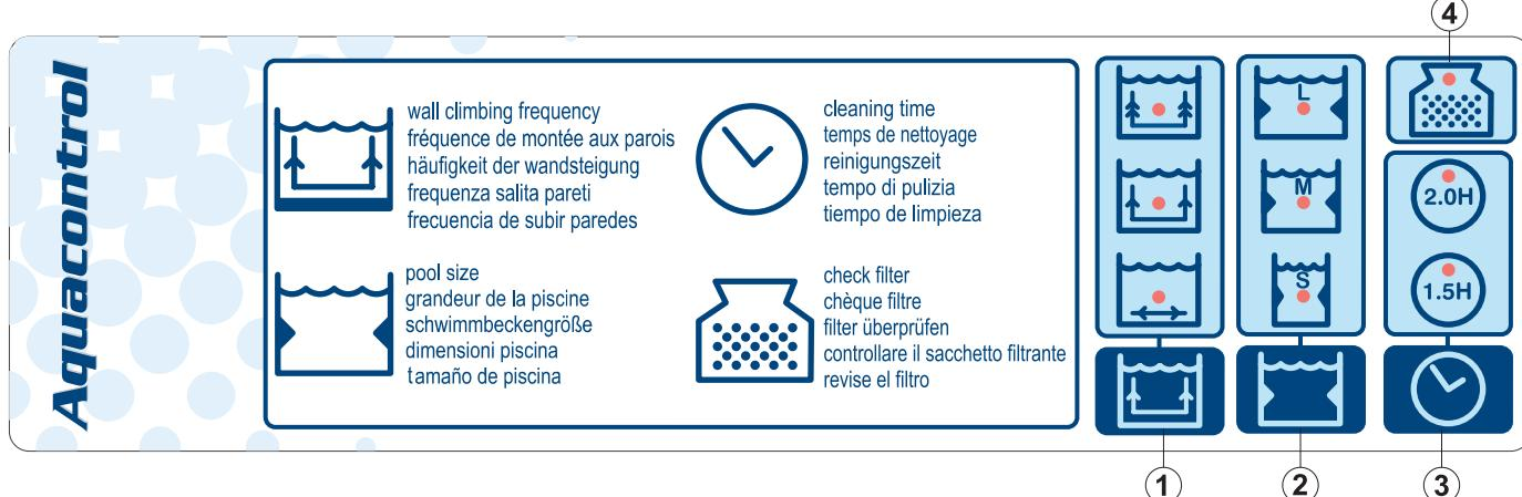
The Aquacontrol is a unique control panel which allows you to communicate directly to the robot and customize it. This human machine interface gives you the option to program different parameters so that the pool can always be cleaned as efficiently as possible. Be sure to select each feature to the best of your knowledge in order to get the maximum lifetime out of the robot. If you prefer not to select any features, the robot will work in default mode and choose the parameters for you.
