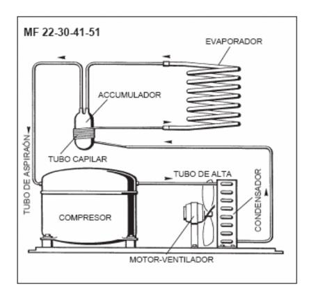
In water cooled models, the high pressure of the system is constant to 8.5 bar in model MF 22, and to 17 bar in models MF 30, MF 41, MF 51 Y MF 61, due to a quantity of water that goes through the condenser, which flow is controlled by the action of the presostate valve that it is open to increase the water flow that cool the condenser.
