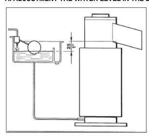
The correct level in the evaporator is 25mm below the outlet ice hole (discharge hole).
