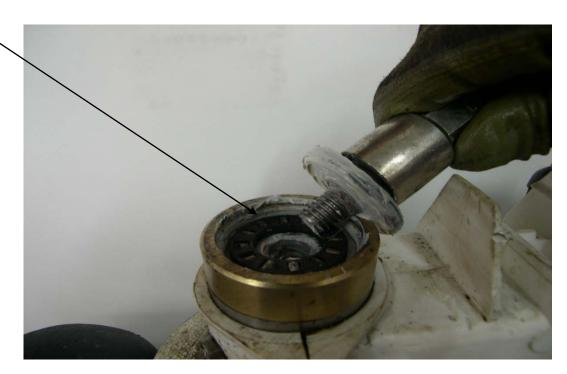
1. CLEAN THE OLD GREASE WITH A RAG AND OIL 6 IN 1, TO GREASE THE BEARING WITH GREASE OF "ALIMENTATION AND WATER REPELENT".
