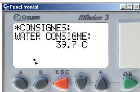
To modify the consignee value, just press the key + or - according to the desired temperature. Once we have modified the temperature, press OK and ESC to come back to the main menu. Available values go from 10°C to 45°C.
