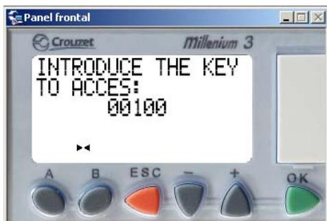
By introducing the password (key) it will be possible to access to the equipment configuration. Contact the Technical service to obtain that
