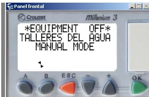
By pushing the keys A – B at the same time the equipment starts working. On the other hand, if we maintain pushed the ESC button during 5 sec the equipment will turn off.
