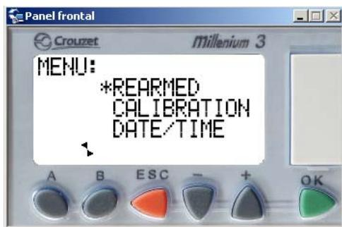
In this MENU we can read the alarms that are active. When activated it will be indicated by means off \* symbol. It will be then necessary to reset the equipment otherwise it will continue blocked. To reset just press – key. Press ESC to leave the MENU
