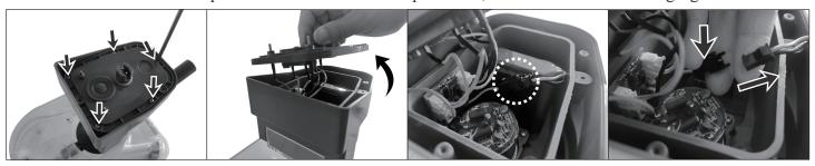
3. After taking out the battery, please wrap the connector with Electrical tape immediately to avoid short circuit caused by contact between two wire terminals.
