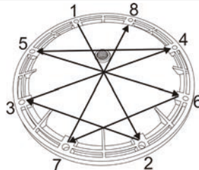
Order for tightening the cover
