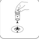
Remove the vial from the sample chamber.
