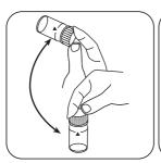
Dissolve tablet(s) by inverting.
