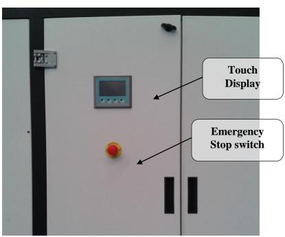
The **control panel** in standard models is mounted on the machine front (depending on model), with the following components (depending on model):
