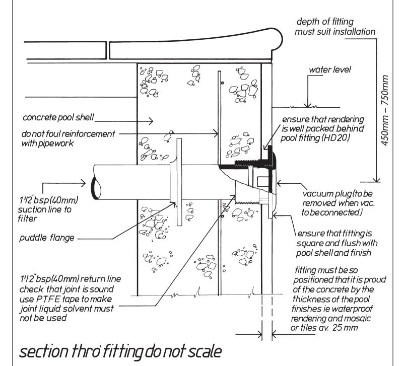
important all pipework and pool fittings must be pressure tested before backfilling and commissioning
