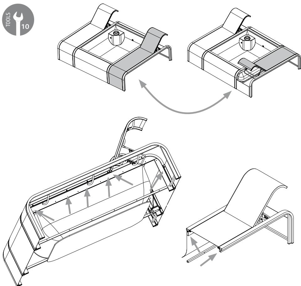
**EN Remove all screws that secure the sheet fastening profiles.**
