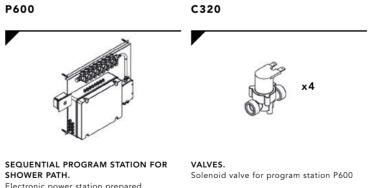
Electronic power station prepared to activate in sequence 8 steps with temporary control of water for each step.Light 1 channel RGB. Complete of Electronic mixer for control temperature. Equipped with keyboard with button to start program with transformer 12 V. Optional aromatherapy during the entire . program. N.B. To be teamed with a single wiring electrovalve C320 12V for each step.
