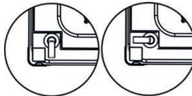
Condensation drainage orientation
