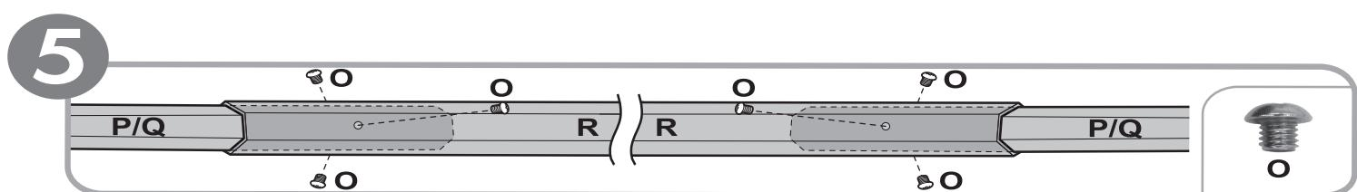
EN To secure the connection of tube "R" with "P"/"Q" inside, tighten three screws "O" in the holes on tube "R" as shown. A minimum overlap of 20cm(8in) is required.
