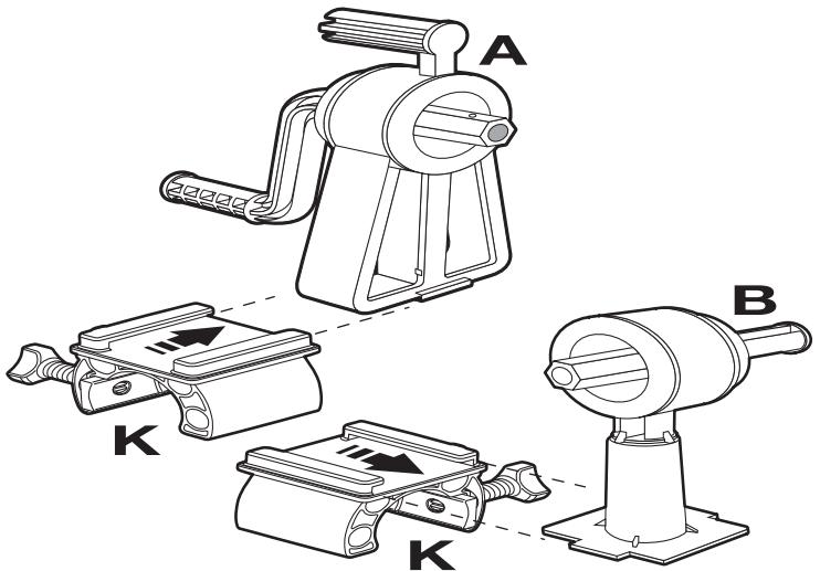
**EN** The required length of the tube set is the length "X" from the inner end of reel support "A" to the inner end of "B", when reel supports are positioned on each side of pool.
