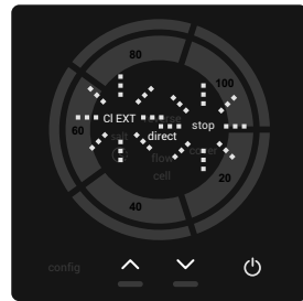
PARADA CLORO EXTERNO Set 0% Led STOP & CL EXT parpadea
