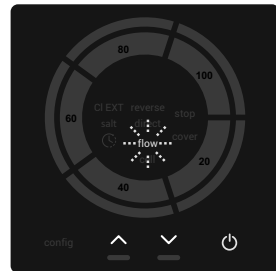
FLOW SWITCH ALARM Led FLOW blinking
