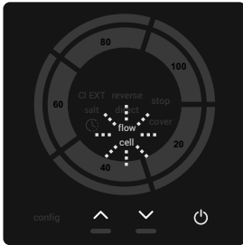
ALARMA FLUJO GAS Leds FLOW & CELL parpadean
