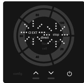
EXTERNAL CHLORINE STOP Set 0% STOP & CL EXT leds blinking
