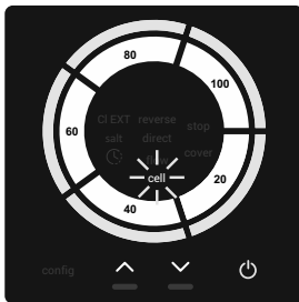
ALARMA CÉLULA Led CELL ON
