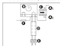
**A**<sub>1</sub>- **A**<sub>2</sub>: Power for the filter pump power contactor coil
