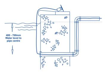
The liner fitting and the liner should be installed as normal. The light body is threaded and shaped in order to be a perfect fit into and over the liner inlet clamp plate.
