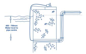
The receiving pipe should be extended/converted to conduit which then runs **above** the water level to create a run for the cable to the central control/power point.
