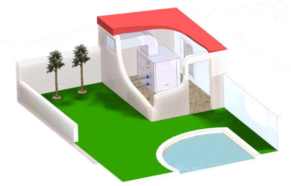
It is necessary to make the duct network so that the air collected by the machine to operate the refrigeration circuit, never return to the machine, and must be expelled to the street. The machine must be located exclusively inside.
