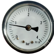
Figure 15 - Reference pressure Pr of 0.8 bar (0.8 kg/cm 2 ) at the start of filter operation.
