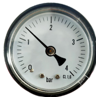
Figure 16 - If the pressure is 0.3 to 0.5 bar higher than the reference pressure Pr: maintenance of the cartridge required
