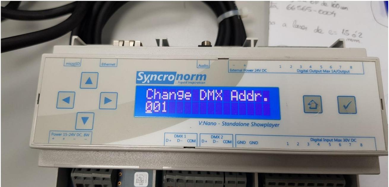
To confirm the address, press the “Check” button to save it.
