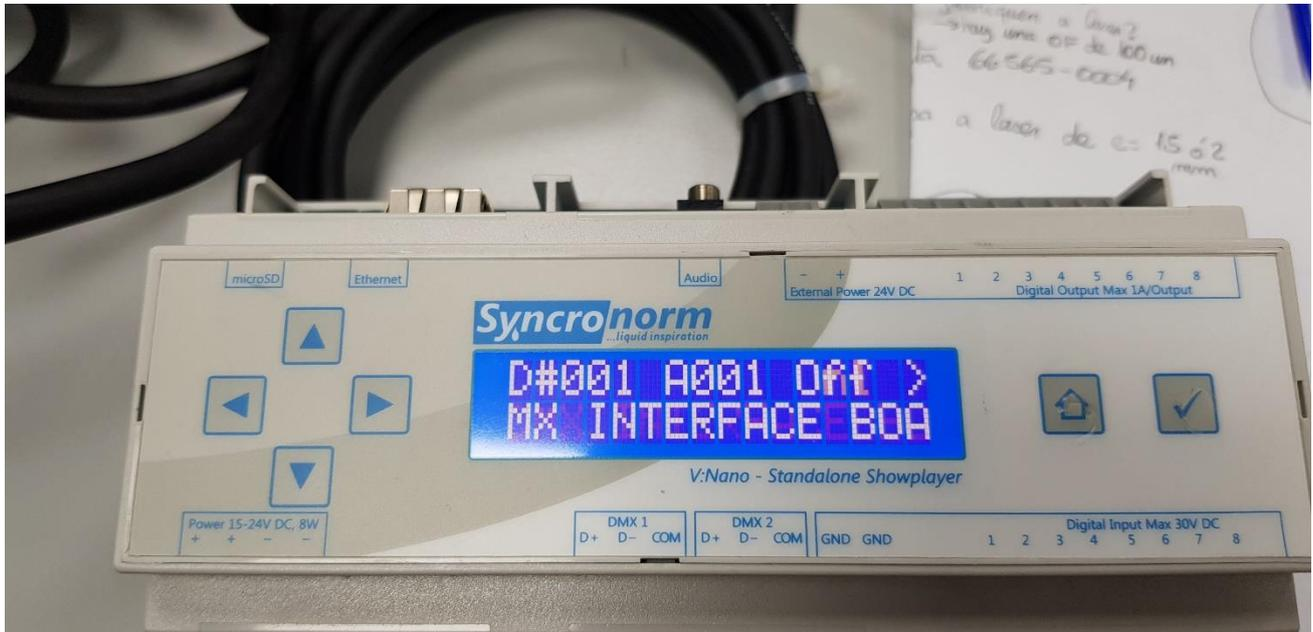
Enter to the desired pump pressing the “Right Arrow” to see the DMX ADDRESS.
