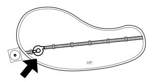
Install at the first hose connection closest to skimmer/or suction line. Ensure correct orientation using guides (Pump/Cleaner) on Leaf Catcher lid.
