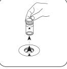
Remove the vial from the sample chamber.
